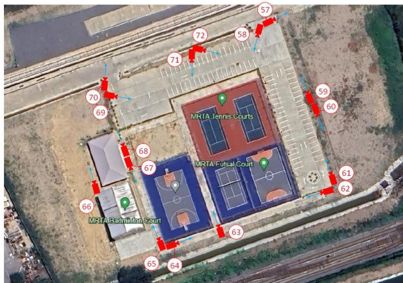
CCTV System Installation at Sport Hall (Outside area)
